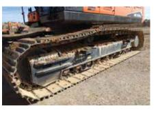
+ Enhanced undercarriage structure. The track chain features sealed, self-lubricating links for long-term dependability, and the track spring and idler are connected for long-lasting performance and easy maintenance.
