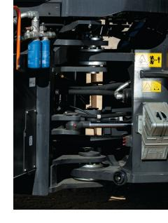
Brakes are located on the outboard side
