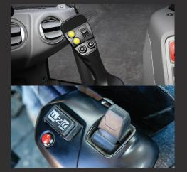
**Joystick Controls** Direction changes don't get any simpler. Just push the joystick buttons to switch between forward, neutral and reverse without even removing your hands from the controls.
