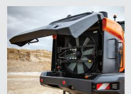
A new radiator with wider fin spacing on some models quickly clears dirt, dust and other large debris to reduce clogging while keeping the cooling system performing consistently – to minimize machine downtime in scrap, forestry and agriculture applications.
